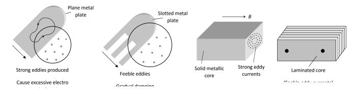
(iii) Application of eddy currents: Though most of the times eddy currents are undesirable but they find some useful applications as enumerated below
