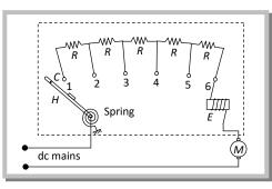
The value of starting resistance is maximum at time t = 0 and its value is controlled by spring and electromagnetic system and is made to zero when the motor attains its safe speed.
