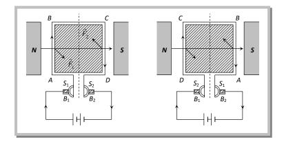
(iii) Working: Force on any arm of the coil is given by  $\vec{F} = i(\vec{l} \times \vec{B})$  in fig., force on AB will be perpendicular to plane of the paper and pointing inwards. Force on CD will be equal and opposite. So coil rotates in clockwise sense when viewed from top in fig. The current in AB reverses due to commutation keeping the force on AB and CD in such a direction that the coil continues to rotate in the same direction.
