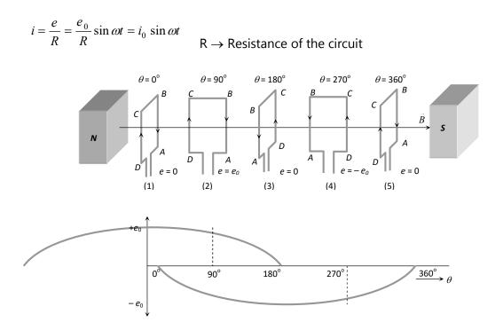
Note: Frequency of ac produced given by  $[f_{AC}] = \frac{NP}{2}$ , where P = Number of magnetic poles of field, N = Rotational frequency of armature coil in rps (rotations per seconds)
