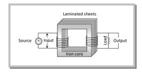
(i) Transformer works on ac only and never on dc.
