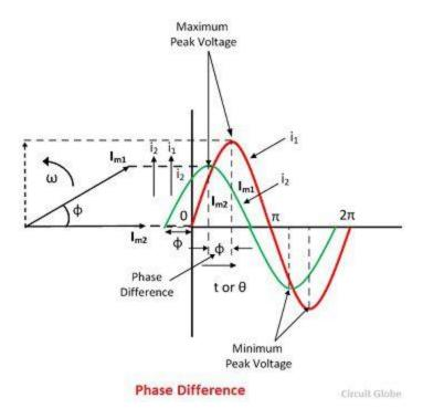
The quantity which attains its +ve maximum value before the other is called a leading quantity, whereas the quantity which reaches its maximum positive value after the other, is known as a lagging quantity. The current  $I_{m1}$  is leading the current on  $I_{m2}$  or in other words, current  $I_{m2}$  is the lagging current on  $I_{m1}$ .
