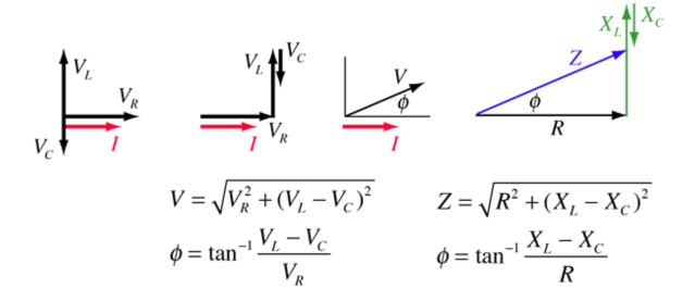
Note that the phase angle, the difference in phase between the voltage and the current in an AC circuit, is the phase angle associated with the impedance Z of the circuit.
