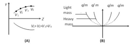
The number of parabola tells the number of isotopes present in the given ionic beam.
