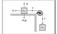
Note: In the above condition Coefficient of friction  $\mu = \frac{m_2}{m_1}$
