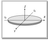
Note: In case of symmetrical two-dimensional bodies as moment of inertia for all axes passing through the center of mass and in the plane of body will be same so the two axes in the plane of body need not be perpendicular to each other.
