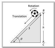
(2) Acceleration in motion: From equation  $v^2 = u^2 + 2aS$
